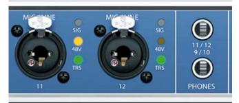
The analog outputs 9 to 12 feed the headphones outputs **Phones 1** and
